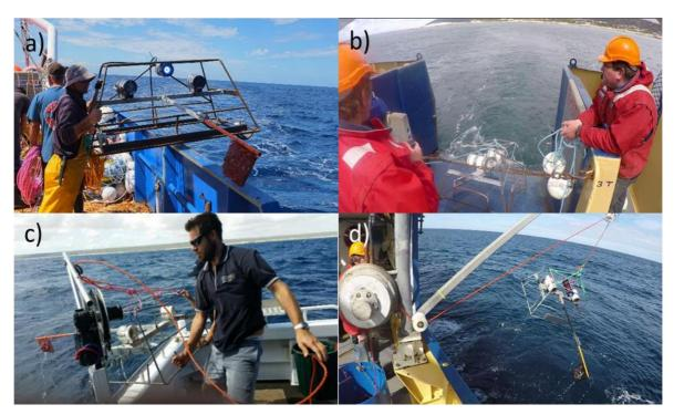
Figure 5.2 a) Deploying a stereo-BRUV from side of vessel. Note that this is a heavy-weight stereo-BRUV setup (Photo: C. Wellingtion/DPIRD). b) Deploying a stereo-BRUV through trawl door on a large vessel. c) Retrieving a standard stereo-BRUV. d) Retrieving a heavy-weight stereo-BRUV off large vessel.
